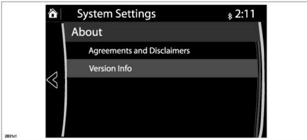
4. Make sure the software version installed in the vehicle is not a later version than the version on MGSS, then select OK. If the software version in the vehicle is earlier than the version on MGSS, update the system using a USB memory stick with the latest software according to the "Reflash Procedure." If needed, refer to "Downloading Update Software to a USB Memory Stick (for additional USB memory sticks)" below.
