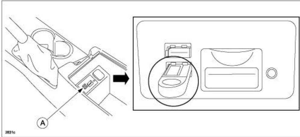
**NOTE:** There should only be the prepared USB memory stick inserted in one of the USB ports. Nothing else should be inserted in the other USB port during the re-flashing process.
