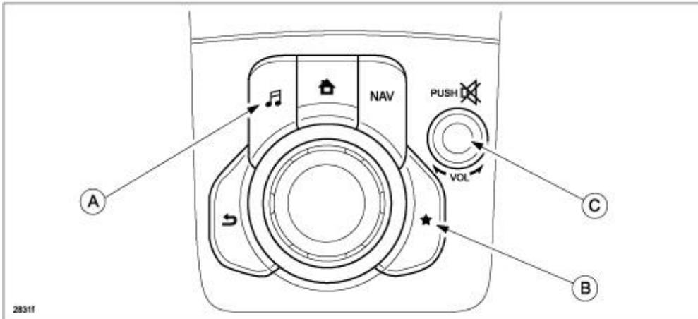
16. Use the touchscreen or the commander switch to input '99' and then select "ENTER" on the Test screen.
