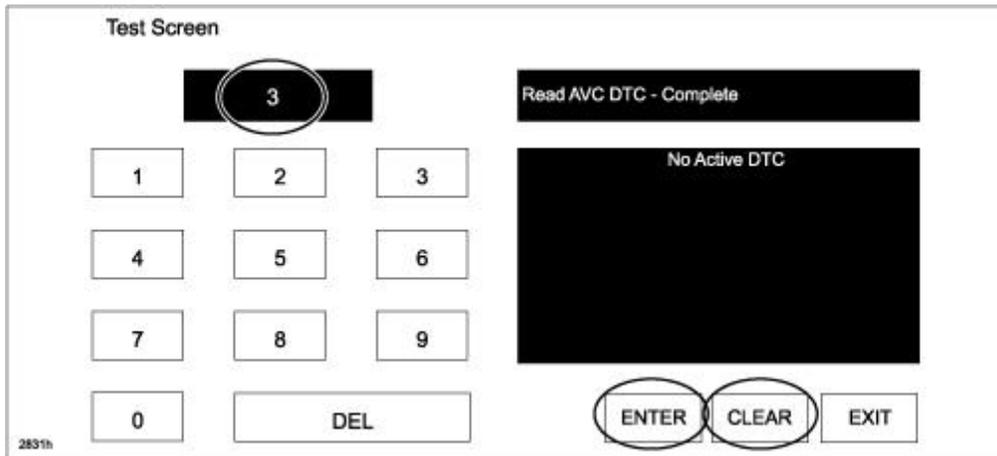
10. Whether any DTCs are present or not, input '2' on the test screen and then select "ENTER". This will internally clear all the earlier set DTCs (in the CMU). Select "CLEAR" to go to next step.
