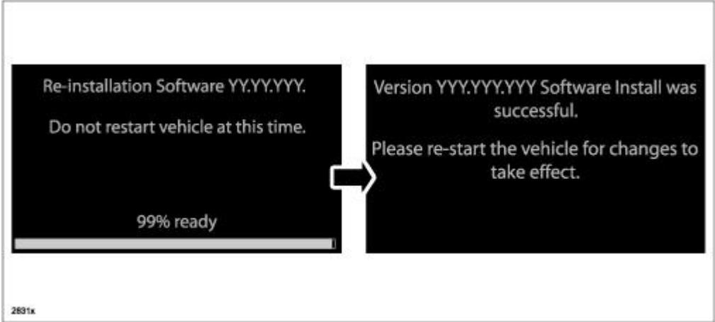
22. After the update is completed with the above right screen, confirm that the push button start indicator light is illuminated (amber) and the display in the instrument cluster is OFF (ignition is in "ACC"). If the ignition is "OFF" and the push button start indicator light is not illuminated (amber), turn the ignition to "ACC" and one of the following two screens will be displayed.
