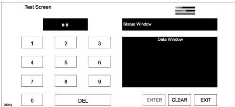
9. On the test screen, input '3' and then select "ENTER" to verify whether any DTCs (in the CMU) are active. Select "CLEAR" to go to next step.
