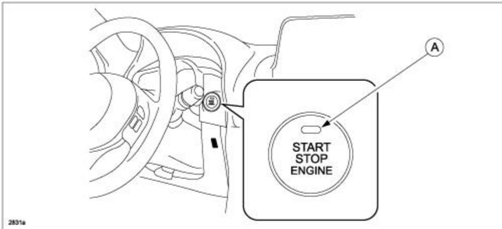
**NOTE:** The engine starts by pressing the push button start while depressing the clutch pedal (manual transaxle) or the brake pedal (automatic transaxle). To switch the ignition position without starting the engine, press the START/STOP ENGINE push button without depressing the pedal.
