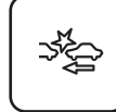
SMART CITY BRAKE SUPPORT (SCBS) INDICATOR LIGHT (RED)/SMART CITY BRAKE SUPPORT (SCBS) WARNING LIGHT (AMBER)
