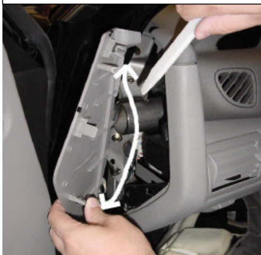
Fig. 5.11 - Wire Path Millenia, IP Side
