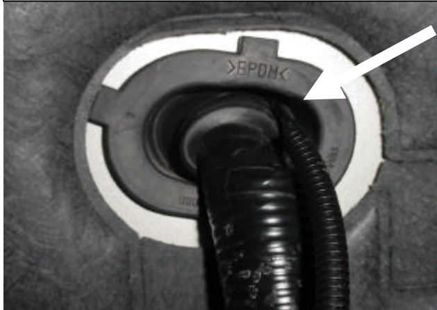
Fig. 4.15 – MPV, Passing Harness Through Dash
