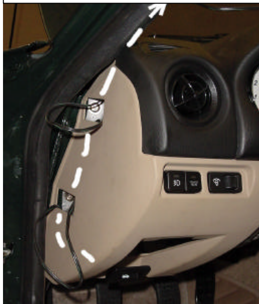
Fig. 5.12 – Wire Path side of Miata Instrument Panel.
