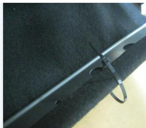
5. Cut off the excess portion of the band shorter than 5mm.
