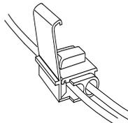
Insert remote start wire into IDC.
