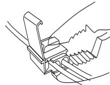
Crimp IDC metal tab over both wires until flush with top of IDC.
