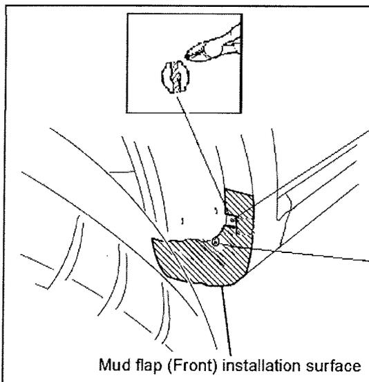
1. Use a soft cloth dampened with IPA (isopropyl alcohol) to clean the surface of the vehicle where the mud flap (front) is to be installed.
