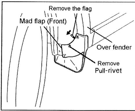
7. Remove pull-rivet and remove the flag over the double-sided adhesive tape backings from the mud flap (front) and affix securely.
