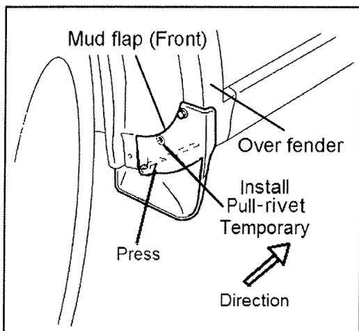
6. Insert pull-rivet without fully installing to ensure proper alignment of mud flap and wheel well.
