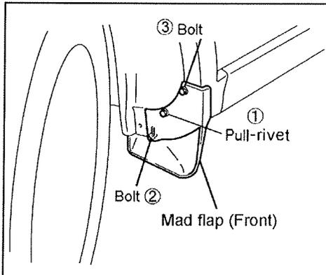
9. Re-Install pull-rivet and torque bolts in order shown in the figure on the left while pressing it against the over fender.
