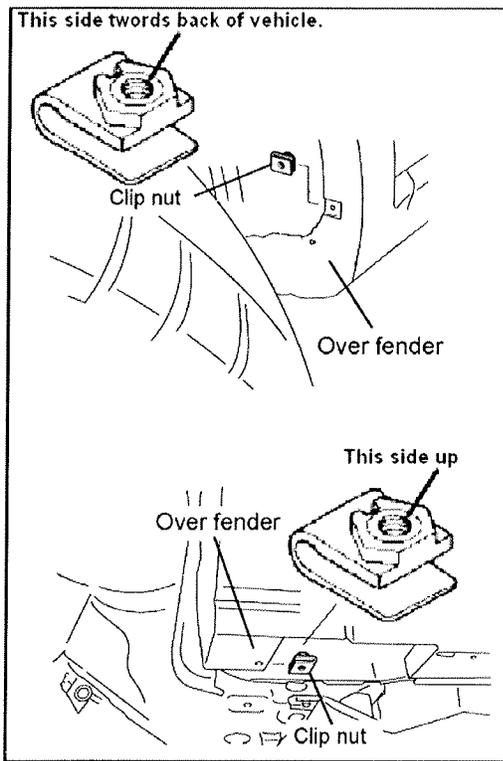
4. Align the clips over fender holes, install the kit clip nuts.
