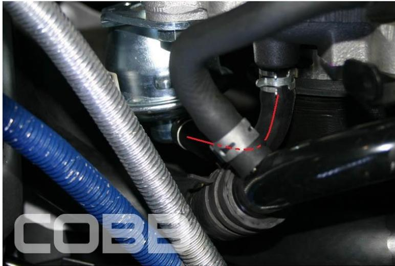
Line 1 which can only be seen from under the chassis plumbs the nipple on compressor outlet to the larger, bottom nipple on the wastegate actuator. This line contains the brass restrictor pill, which is actually pressed inside the compressor housing nipple. This is a view from the bottom of the turbocharger.
