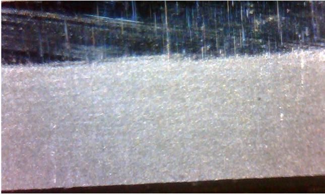
**Figure 3.** Coating formation (bottom strip) on cylinder ring. Formation of the DLC layer eliminates surface scratches, visible on upper portion of the ring.
