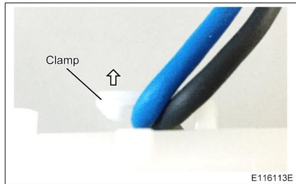
5. Remove the connector of the wire harness (with the flange).
