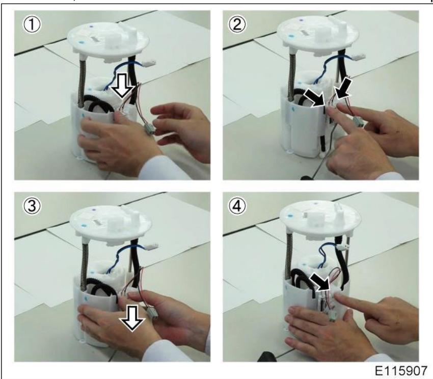
Make sure that the lock has been checked and secured.
