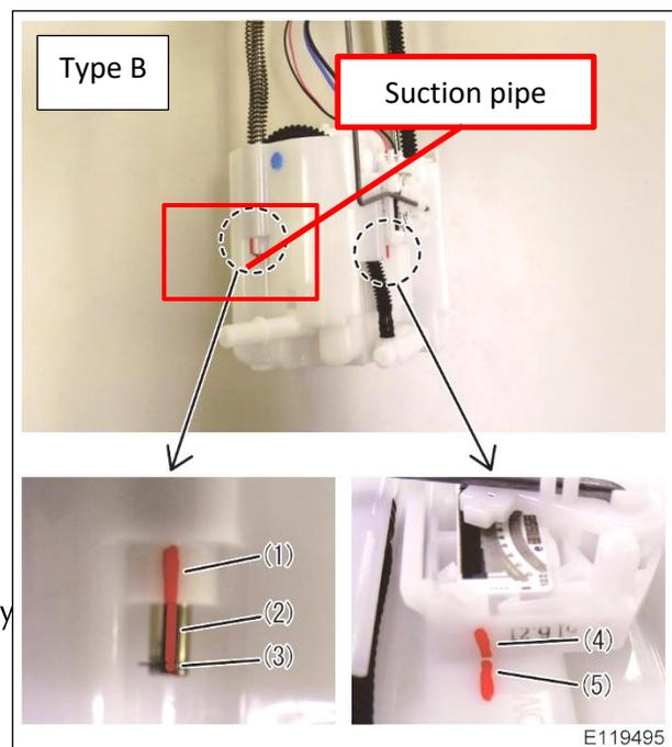
Type B has the valve referred to in the tube routing diagram.
