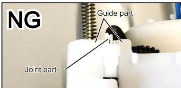
Check the joint part is in the correct
