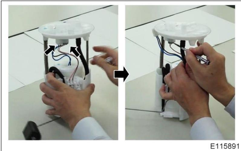
6. Remove the fuel gauge sender.
