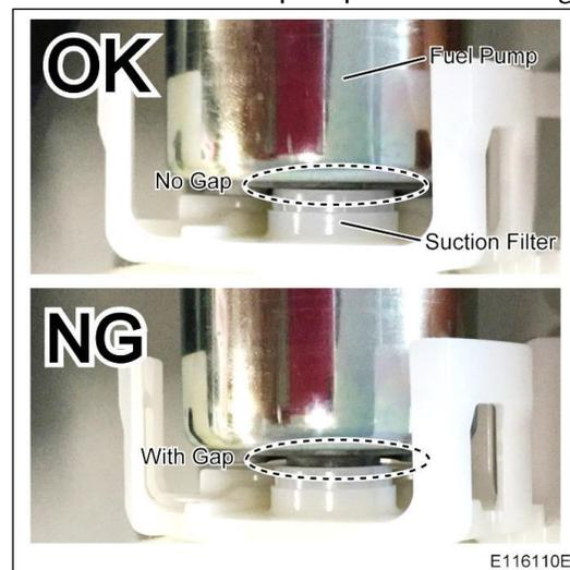
2. Install the new spacer, new O-ring, and wire harness to the new fuel pump.
