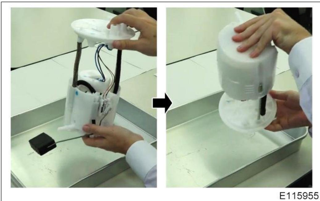
2. Mark the (1) rod guide, (2) rod, (3) E-ring, (4) fuel gauge sender and (5) reservoir cup with a marker before disassembly to avoid re-assembling incorrect.
