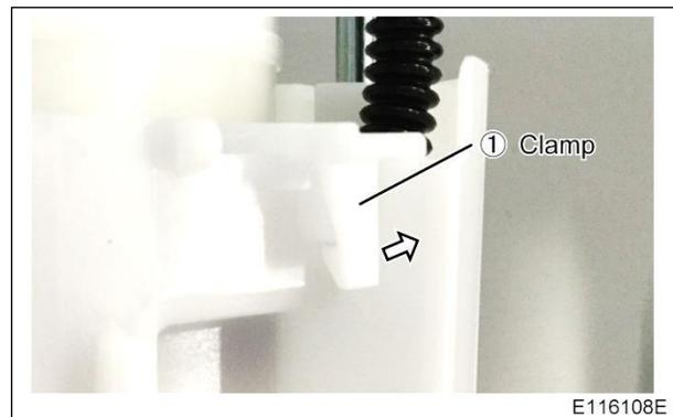
9. Pull out the high-pressure pump from the reservoir cup.
