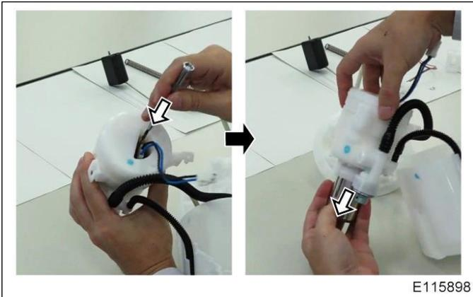
13. If the O-ring remains on the high-pressure pump, use a long hook-like rod to remove it while ensuring that the O-ring seal is not damaged.
