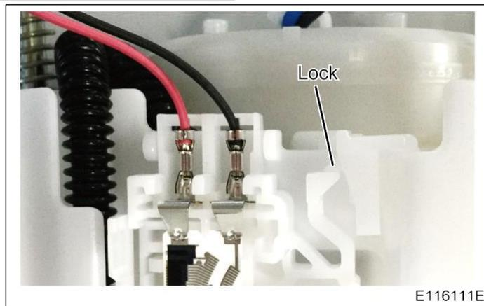
6. Install the connector of the wire harness. Make sure that the lock has been checked and is secure.
