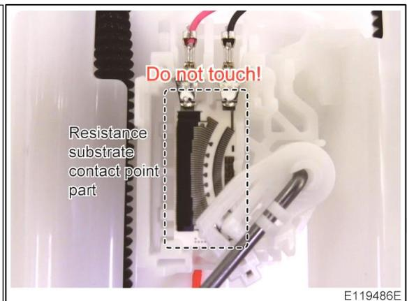
Remove the jet pump from the reservoir cup. (Only 4WD that has fuel pump# PYY2 has transfer jet pump)
