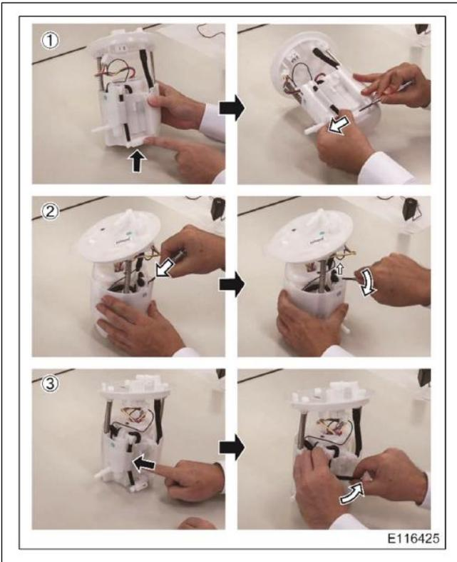
① Remove the jet pump for pumping.
