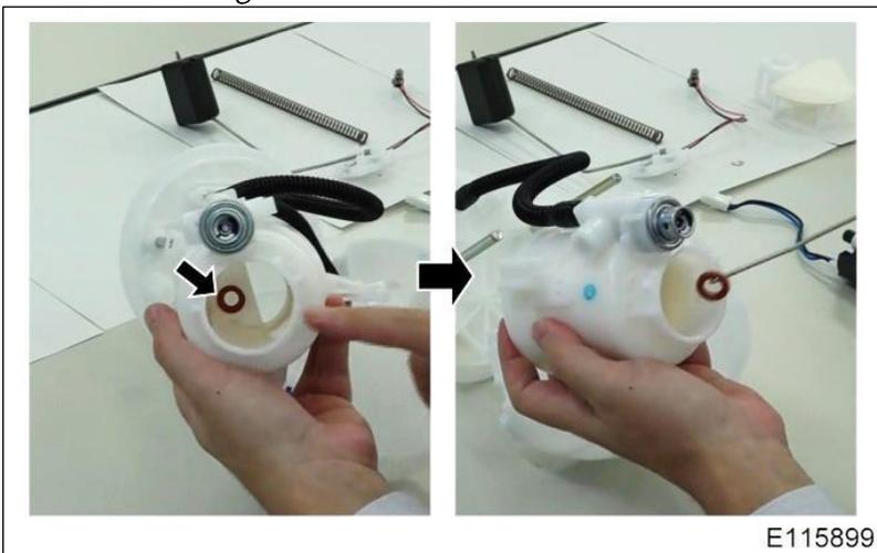
14. Remove the wire harness and spacer from the fuel pump.
