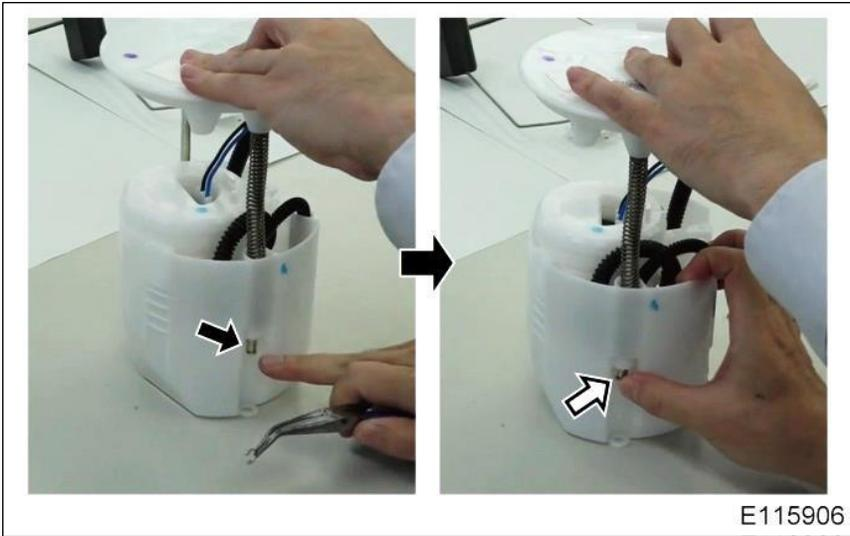
5. Install the fuel gauge sender in the reservoir cup.
