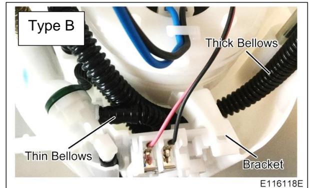
4. Remove the wire harness from the clamp. Spread the clamp and remove the wire while ensuring that the wire harness is not damaged.
