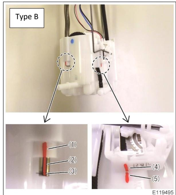
3. Check the routing condition of the wire harness and tube. The routing is the same during reassembly.
