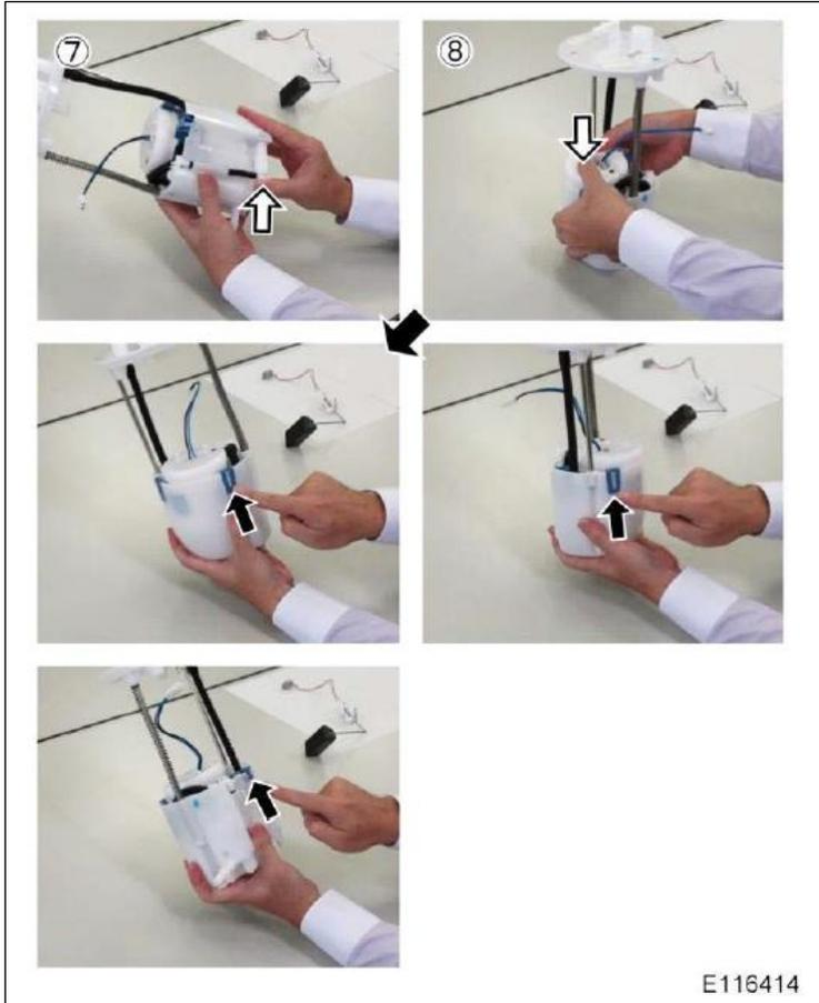
⑦ Install the jet pump on the reservoir.
