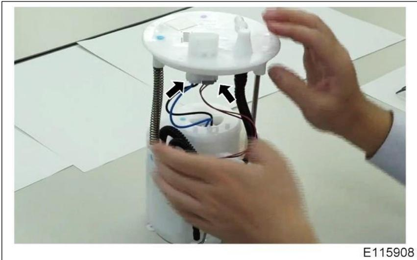
7. Install the wire harness in the clamp section.
