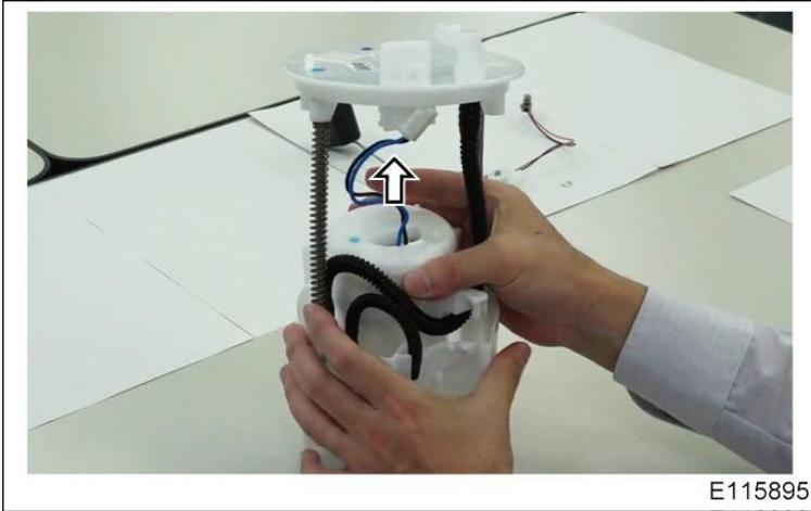
10. Remove the spring from the rod with the spring on it.
