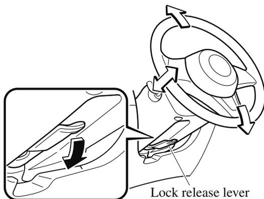
2. Tilt the steering wheel and/or adjust the steering column length to the desired positions, then push the lever up to lock the column.
