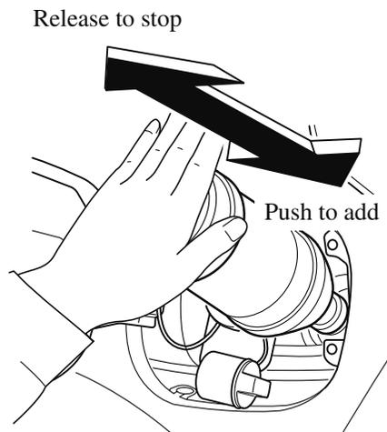
8. Remove the bottle in the reverse order of the insertion. At this time, be careful of DEF dripping from the bottle.
