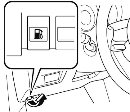
2. To remove the fuel-filler cap, turn it counterclockwise.
