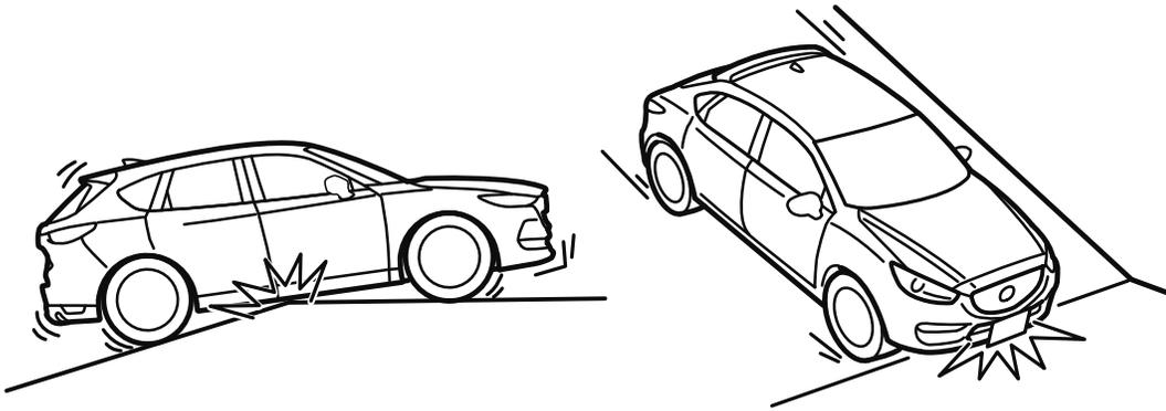
This vehicle is equipped with low profile tires allowing class-leading performance and handling. As a result, the sidewall of the tires are very thin and the tires and wheels can be damaged if driven through potholes or on rough/uneven roads at excessive speeds. Use care and reduce speed when traveling on rough/uneven roads or through potholes.
