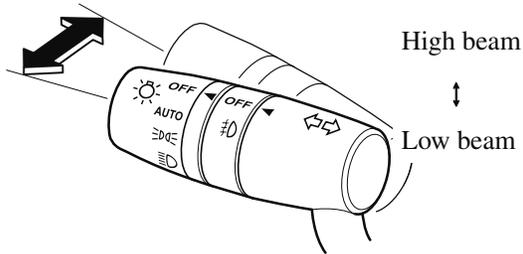
When the headlight high-beams are on, the headlight high-beam indicator light is turned on.
