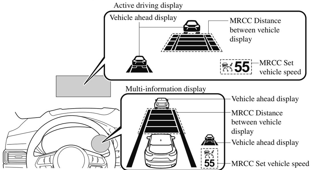
If there is a problem with the MRCC with Stop & Go function system, a message is displayed on the multi-information display. Check the center display to verify the problem and then have your vehicle inspected by an Authorized Mazda Dealer.
