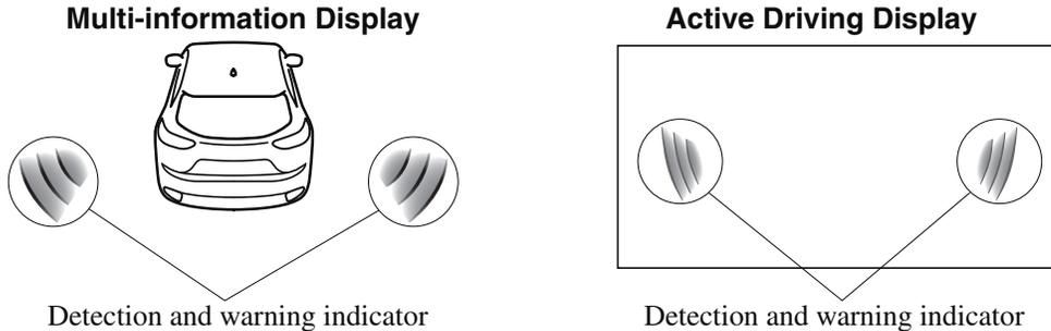
The detected direction is displayed with a detection indicator (white) when an approaching vehicle is detected. In addition, if the turn signal lever is operated to signal a lane change while the vehicle is detected, the display changes the color (amber) of the warning indicator.
