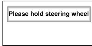
*If the steering wheel is held lightly, or depending on the road conditions, the system may detect that you have released the steering wheel (not holding the steering wheel) even if you are holding it, and display a message in the multi-information display or the active driving display.*
