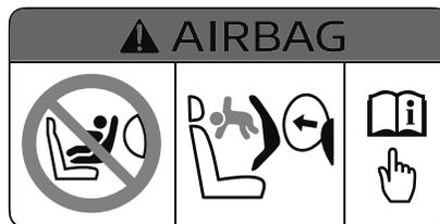
**Do not install a front-facing child-restraint system on the front passenger seat unless it is unavoidable:**
