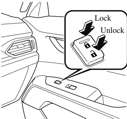
To lock all the doors and the liftgate from an open front door, press the lock side of the door lock switch and then close the door.
