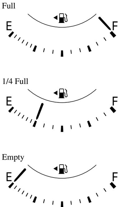
If the low fuel warning light illuminates or the fuel level is very low, refuel as soon as possible.
