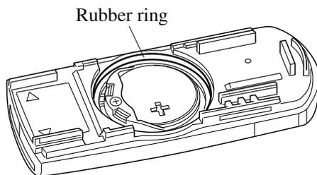
6. Insert a new battery with the positive pole facing up, and then cover the battery with the battery cap.
