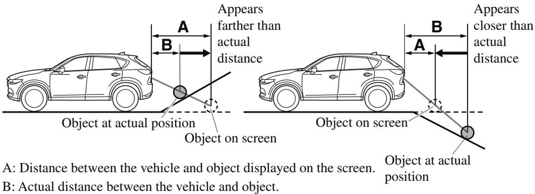
A: Distance between the vehicle and object displayed on the screen.
