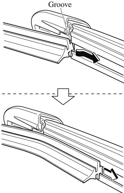
6. After pulling the blade rubber in the direction of the arrow and sliding the blade rubber to a position to check the blade holder groove, slide the blade rubber end in the opposite direction.
