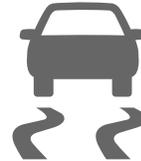
This indicator light stays on for a few seconds when the ignition is switched ON. If the TCS or DSC is operating, the indicator light flashes.
