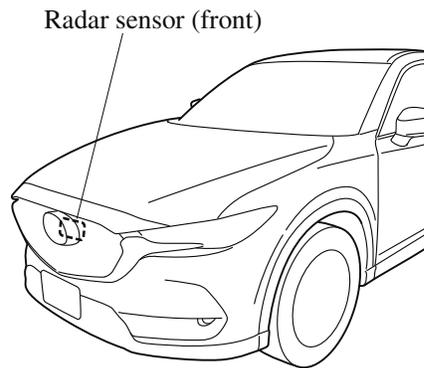
If “Front Radar Sensor Blocked” is displayed in the multi-information display of the instrument cluster, clean the area around the radar sensor (front).
