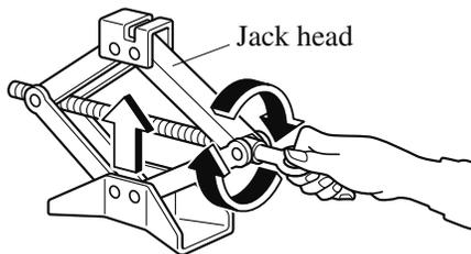
5. Place the jack under the jack-up position closest to the tire being changed with the jack head squarely under the jack-up point.
