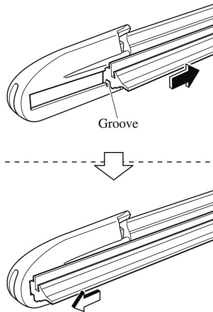
7. Make sure that the blade rubber is correctly installed to the blade holder.
