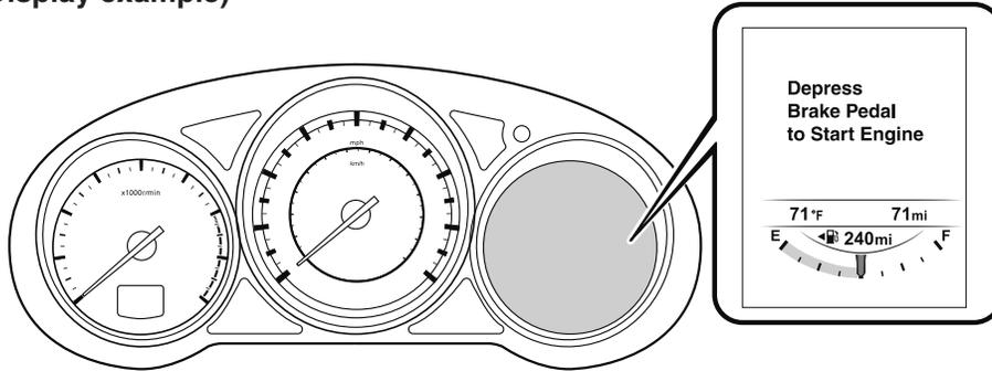
If the warning light turns on/flashes simultaneously or a symbol is indicated in the display, check the information regarding the warning light or symbol. Refer to If a Warning Light Turns On or Flashes on page 7-24.
