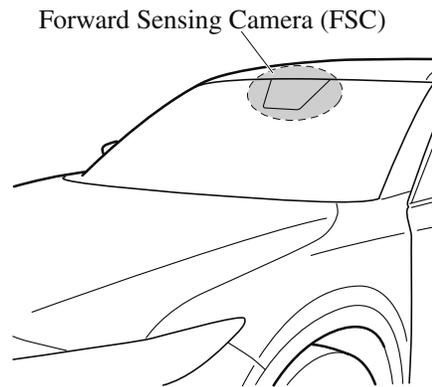
The Forward Sensing Camera (FSC) determines the conditions ahead of the vehicle while traveling at night and detects traffic lanes. The distance in which the Forward Sensing Camera (FSC) can detect objects varies depending on the surrounding conditions.
