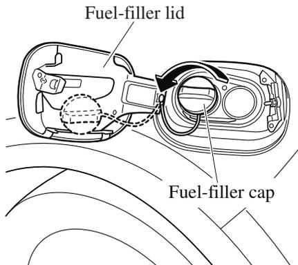
4. Insert the refueling nozzle all the way and begin refueling. Pull out the refueling nozzle after the refueling stops automatically.
