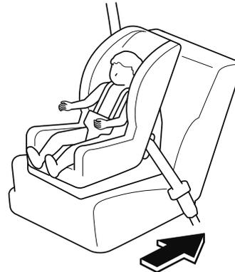
3. Remove the head restraint. However, when installing a backless booster seat, always install the vehicle head restraint to the seat where the backless booster seat is installed.
