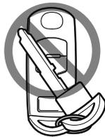
➤ Spare keys or keys for other vehicles equipped with an immobilizer system touch or come near the key.
