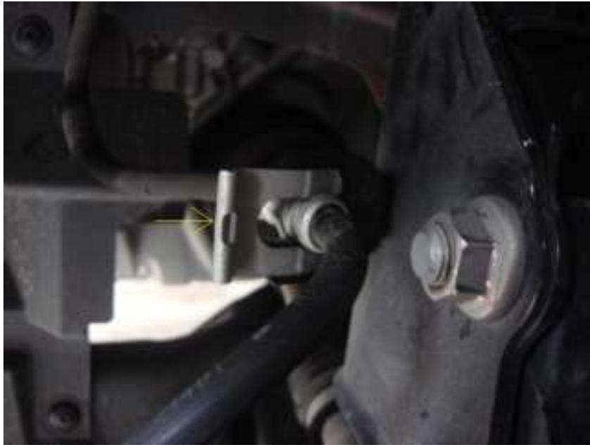
8. Remove brake hose clip by pulling towards the front of the vehicle using a pair of pliers (see yellow arrow for direction of pull (I already loosened the clip, hence the use of my
