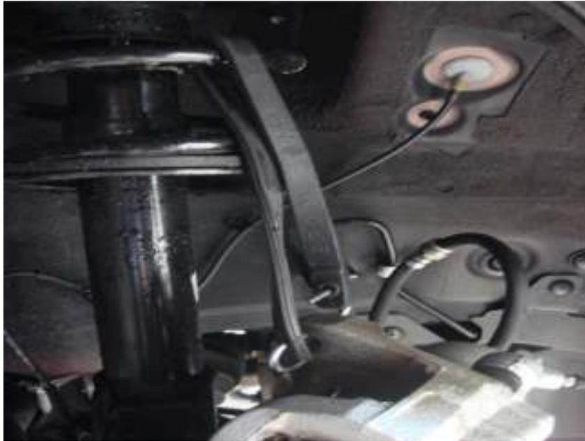
***Note:*** *If the caliper is hanging-up on the rotor due to the pads contact with it, wiggle it side to side with force to slightly push the pads in and create space between rotor and pad.*
