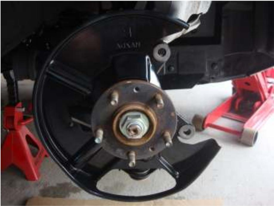
16. Before installing the new rotor, compare it with the old (OEM) one for compatibility (holes line-up, same size, thickness,
