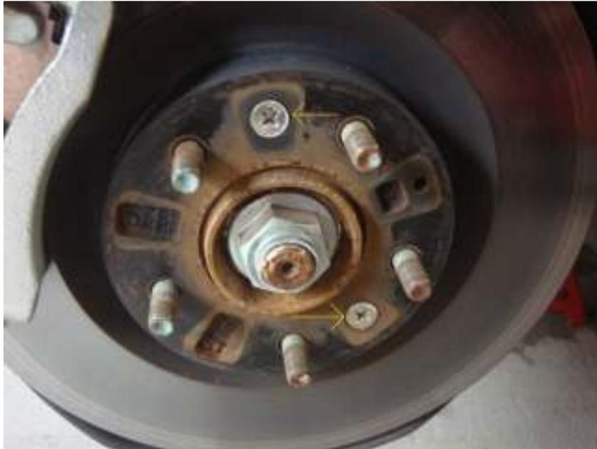
14. Rock the rotor back and forth to loosen it from the hub. **Note:** *Anticipate the full weight of the rotor (approx. 18lbs., maybe more) as it separates from the hub. Be careful not to drop it on the ground, or worse on any part of your body.*
