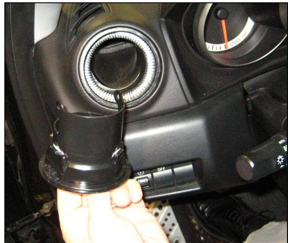
2. Position your hands/fingers as per the illustration below and apply some outward force. While still applying this force, slowly rotate the inner vent receptacle counter clockwise (there is an internal alignment tab which will prevent you from removing this component unless properly aligned). The moment the slot and tab are aligned, the vent receptacle will easily “pop” out of the dash.
