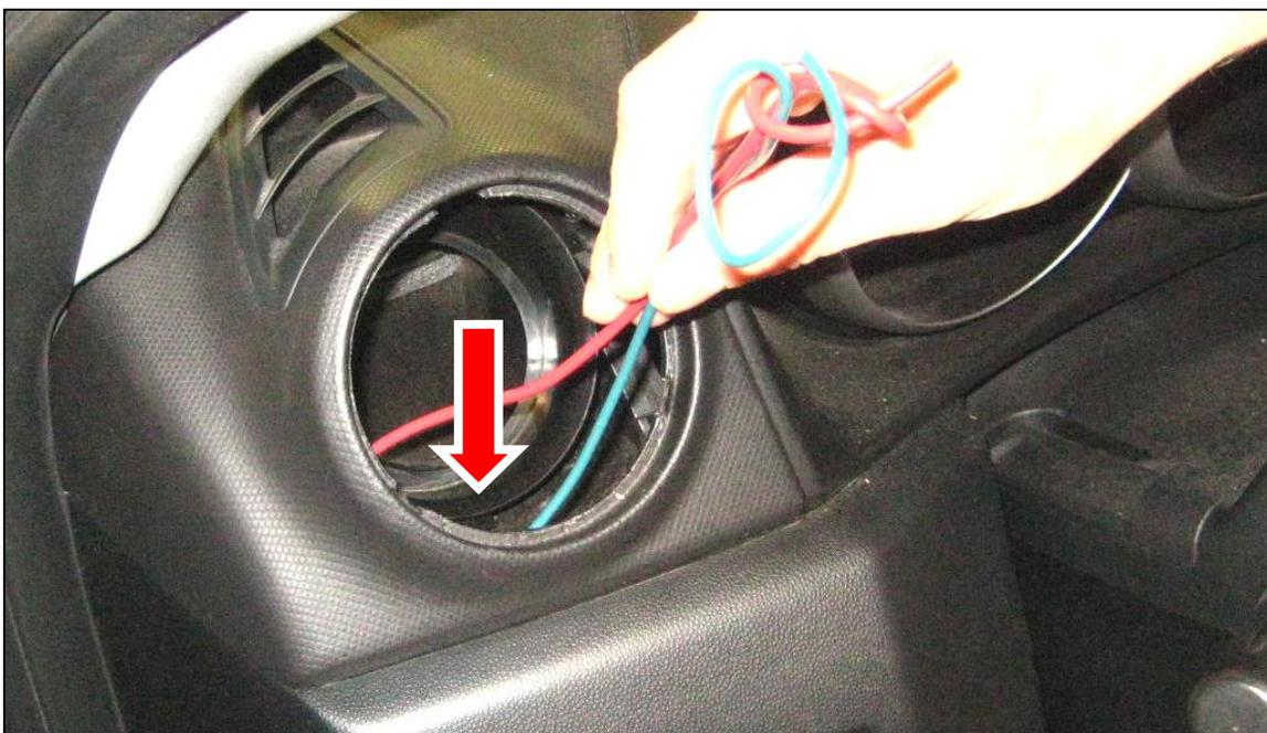
4. Feed the wiring through the VentPod and install the VentPod into the dash (see note below). Ensure the wires are routed through the slot, and the slot is positioned facing the footwell. Make all necessary wiring connections with the gauge as per the gauge manufacturer's recommendations.
