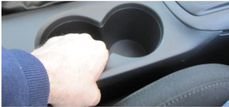
Open the center console and lift the rear edge of the cup hold trip as shown.
