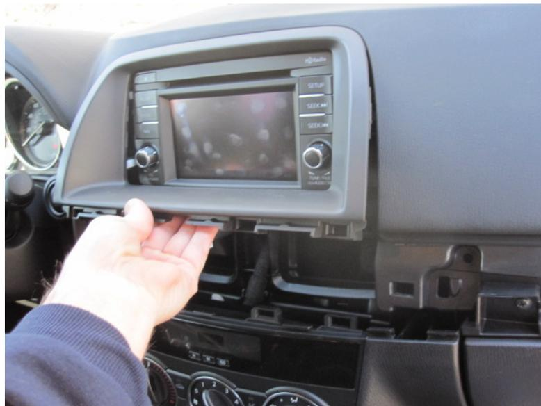
To remove the head unit, there are two Phillips screws (one on the left and right), and one 10 mm bolt on the bottom that need to be taken out.
