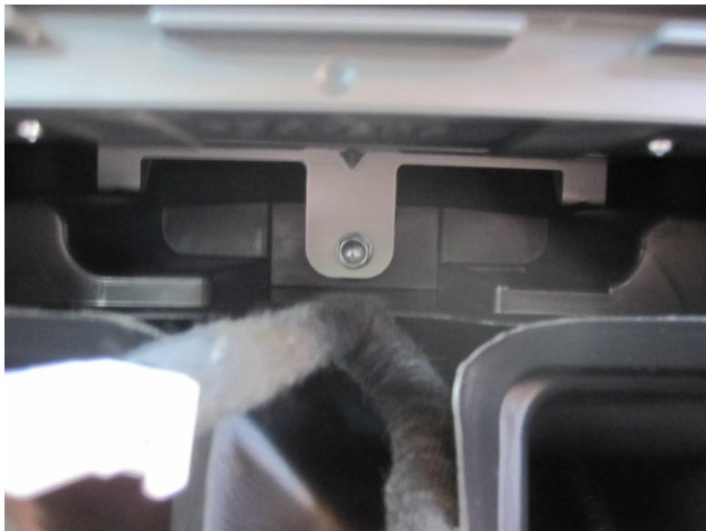
At this point, you simply grab the head unit and pull it straight out. You will have to remove the connections on the back once the head unit is far enough out to reach them.
