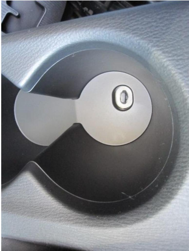
To make wiring access easier, you should also remove this bracket in front of the shifter. Simply remove the two Phillips screws and take it out.
