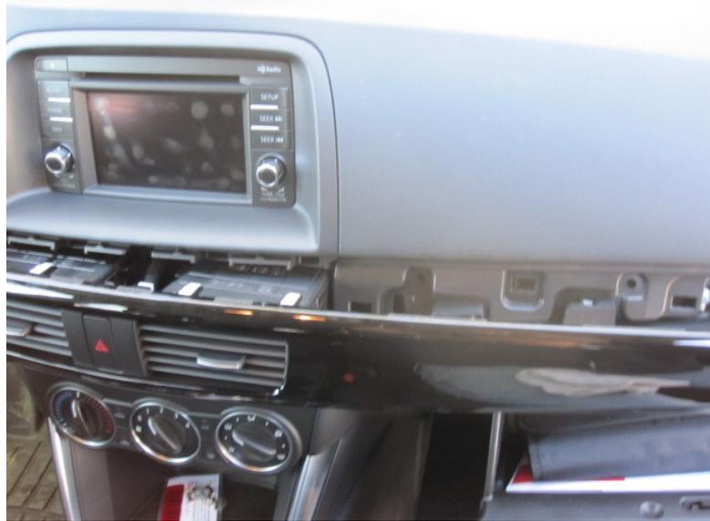
Next, remove the stereo head unit trim by grasping and pulling the bottom as shown here, then just work it off the rest of the way. It is only held on with clips, the same as the trim piece we already removed.
