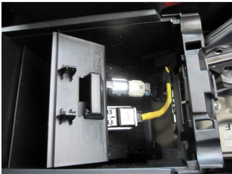
To remove the port itself, there are two clips that push in on both sides of the port. I found the easiest way was to push in the two on one side, slide them through, then repeat for the other side.
