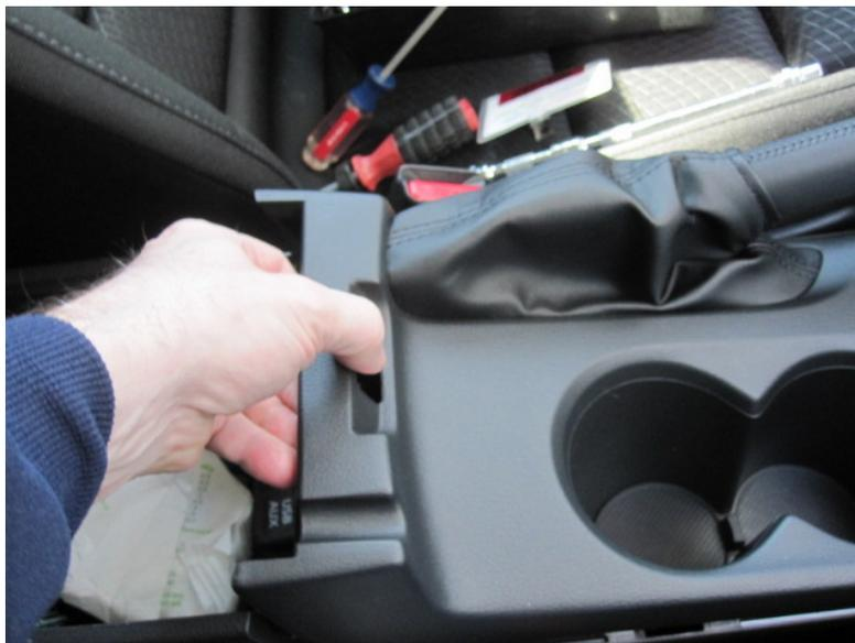
Continue to work your way around to the drivers side of the trim. Once you have it all loose, carefully lift the whole piece and slide it up and off of the lifted parking brake handle. You will need to gently bend the front of the trim where the storage cubby is in order to get it all the way off. The trim has a 'hinge' there to facilitate this. Do not force it in any way or you may break something.
